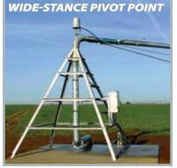
Standardized dimensions to retrofit many existing pads. Constructed with extra cross-ties to support spans up to 203.5'. Features include galvanized removable elbow and Pierce Conduit Seal.
