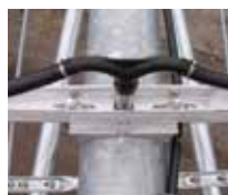
The Senninger Double Gooseneck attaches to the 3/4" x 4" galvanized nipple through a pre-drilled hole in the aluminum channel and into an existing outlet.
